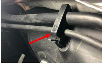
STEP 6: Remove the fuel line quick disconnects. Disconnect the sending unit electrical connector.
